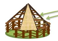
Step Eight: Place two wood "rings connecting the rafters.
